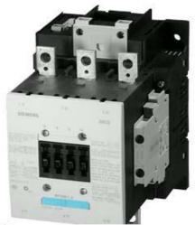
CONTACTOR, 90KW/400V/AC-3, AC(40...60HZ)/DC OPERATION UC 21...27.3V AUXIL. CONTACTS 2NO+2NC 3-POLE, SIZE S6 BAR CONNECTIONS ELECTRONIC OPERATING MECHANISM WITH 24V DC PLC INTERFACE SCREW TERMINAL
